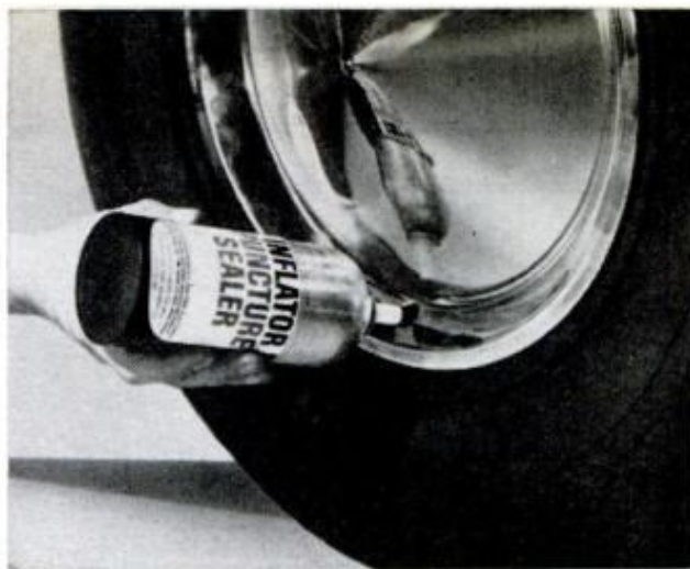
AEROSOL PUNCTURE SEALERS are fine in emergency; drive or spin wheel so sealer is distributed evenly
